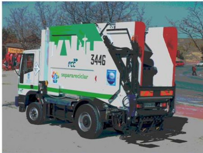
2 Axle vehicle, configuration 4x2 maximum width reduced to 1.8 metres and GVW 12 tons (4 units)
